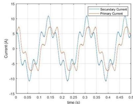
Fig. 5 Voltage and current of primary and secondary with  $k_3=0.1$ ,  $k_5 = 0.2$  and  $k_7 = 0$
