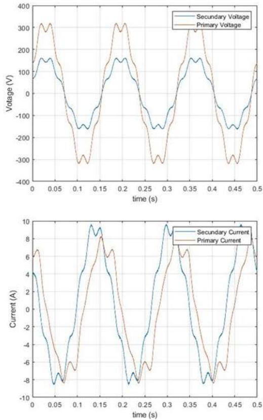
Fig. 6 Voltage and current of primary and secondary with  $k_3=0$ ,  $k_5=0.1$  and  $k_7=0.1$
