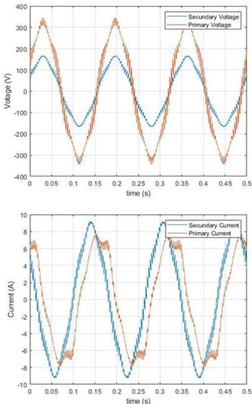
Fig. 7 Voltage and current of primary and secondary with high orders
