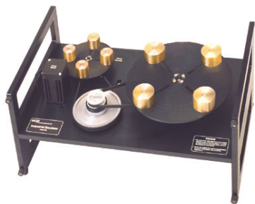
Figura 2. Emulador Industrial, Modelo 205 da Educational Control Products (ECP) (ECP, 2000).
