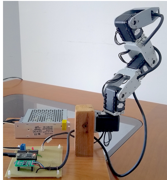
Figure 2. Didactic manipulator used in this work.
