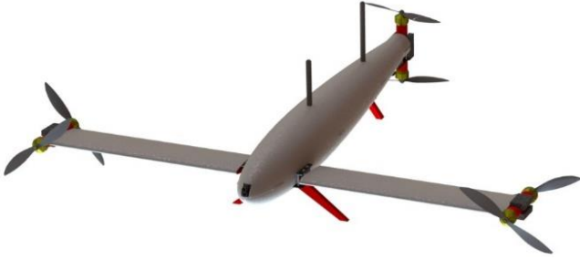
Fig. 4. Aircraft's 3D model in a symmetric configuration.
