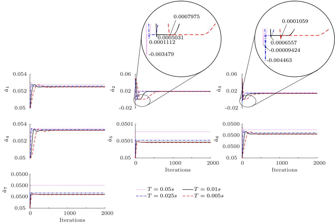
Figure 2: Estimated parameters in ACPP for four different sampling periods. For  $T = 0.05s$  there are two negative parameters, for  $T = 0.025s$  there is one negative parameter, and for  $T = 0.01s$  and  $T = 0.005s$  all parameters are positive.
