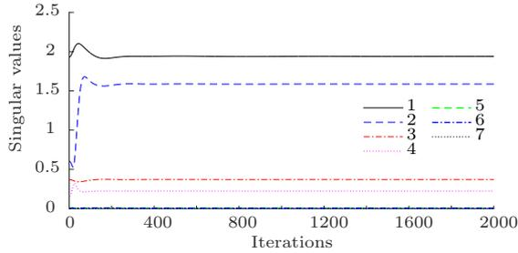
Figure 5: Singular values related to each robot's joint during the simulation of the IDFL. Since the last three singular values are much smaller than the largest one, the resultant torque related to the last three joints are almost inexpressive compared to the dominant torque.
