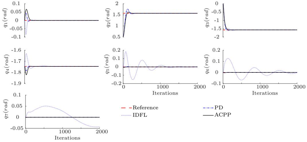
Figure 4: Joints configurations during simulation. For the IDFL, the last two joints did not reach the desired values due to the difference in the singular values of the JSIM (i.e., JSIM had a large condition number near the desired configuration).
