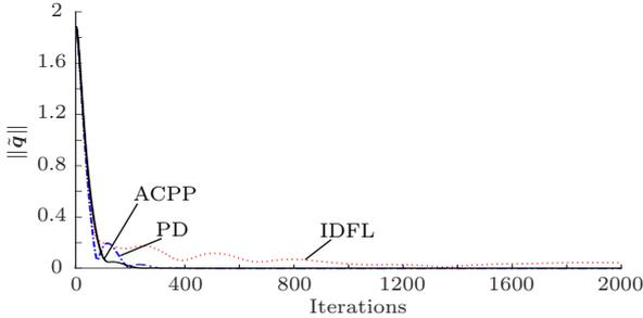
Figure 3: Norm of the vector of joints error. The adaptive controller with positive parameters (ACPP) presents the smoothest decay among all compared controllers.
