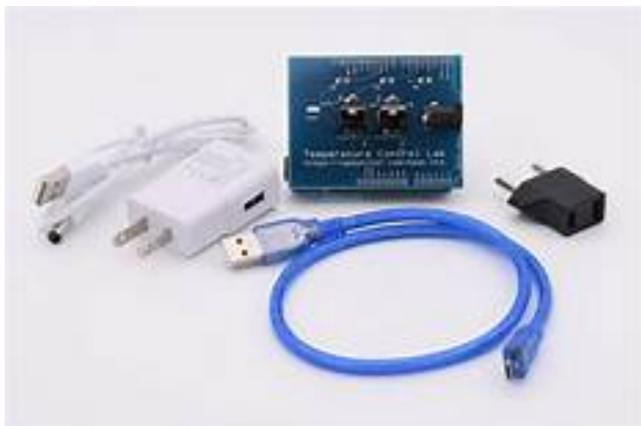
Figure 1. TCLab components: Arduino Leonardo, Thermal system shield, USB cable, External power source
