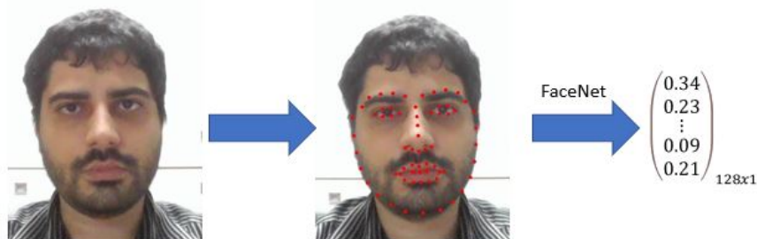
Figure 5. Vectorization process from facial point detection using HOG and FaceNet.
