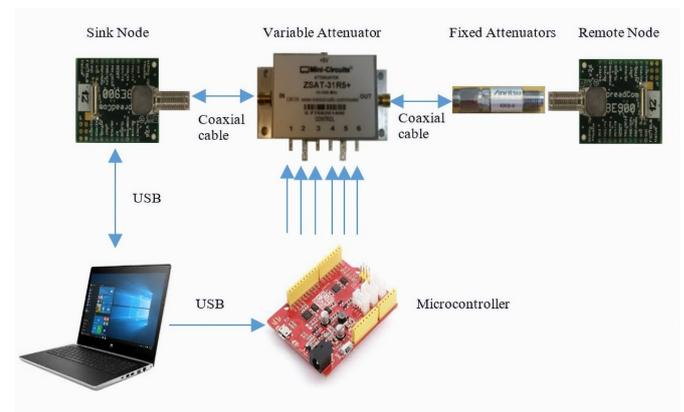
Figure 1. The workbench components and connection setup.
