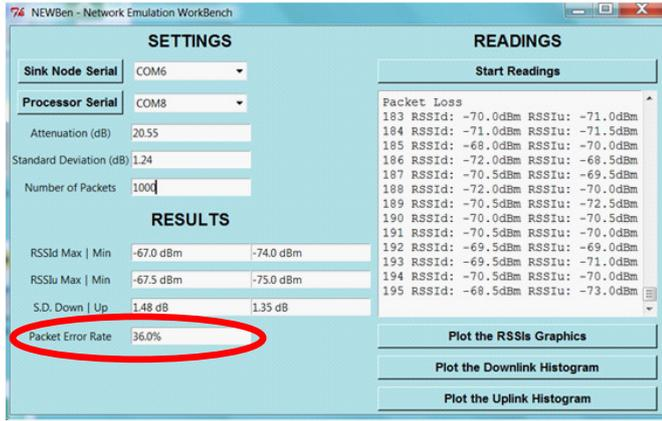
Figure 2. The HMI showing the settings and results menus. The obtained PER for 250 Kbps is circled in red.
