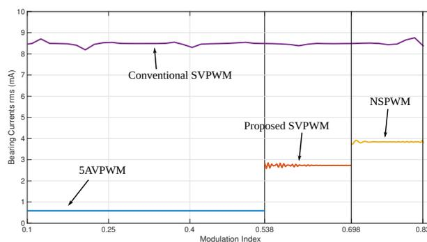
Figure 13. Proposed SVPWM, 5AVZPWM, NSPWM and Conventional SVPWM comparison regarding bearing current.
