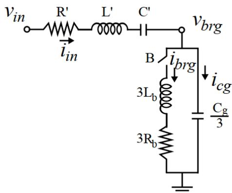
Figure 11. Bearing currents model shown in Chen et al. (1996).
