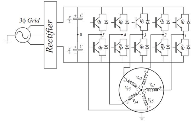
Figure 1. Five-phase machine drive system.
