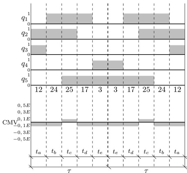
Figure 10. CMV voltage for proposed SVPWM, sector I.
