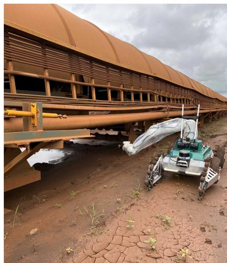
Fig. 1. Robotic inspection of a belt conveyor.
