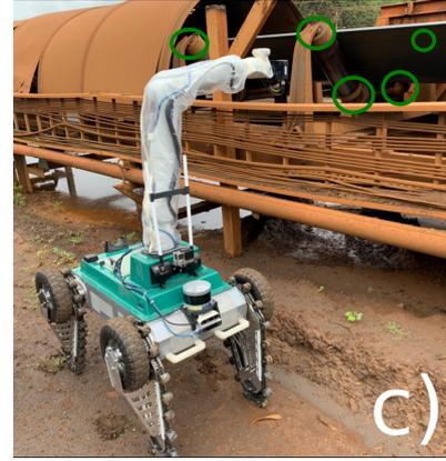
Fig. 2. From the robot position, any of the rollers could be the source of the noisy sound.
