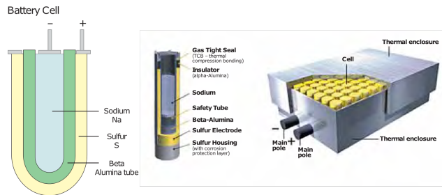
Figure 1. Construction principle of the Sodium/Sulfur battery(5).
