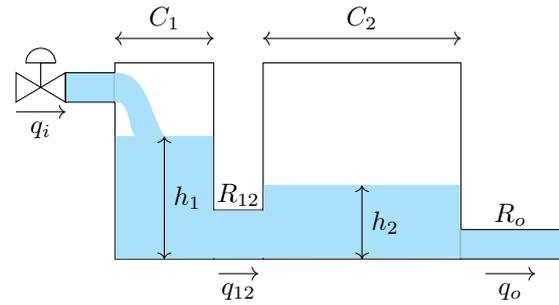
Figure 2. Interacting tank system.
