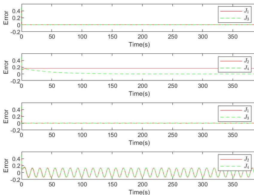
Figure 5. Transient responses of the error between plant and model outputs for the structure with (dashed) and without (solid line) integral control when load disturbance of amplitude 0.8 (top two panels) and sinusoidal disturbances of amplitude 1, frequency 0.5 rad/s, (bottom two panels) are applied.
