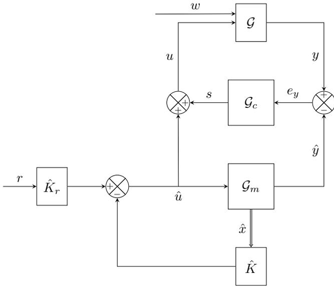
Figure 1. Reference model control with dynamic output feedback. The reference model performance is governed by a full state feedback control, using the gain  $\hat{K}$ . The plant,  $\mathcal{G}$ , under the action of disturbances signals,  $w$ , must follow the output of the reference model,  $\mathcal{G}_m$ . This task is accomplished by the second degree of freedom, provided by the dynamic output feedback controller,  $\mathcal{G}_c$
