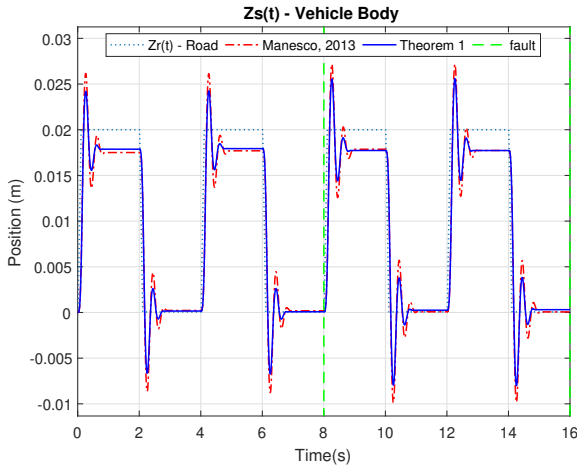
Figure 5. Active Suspension System behavior with Switched Control via Output Feedback and robust SOF controller Manesco (2013) closed-loop (0-8s); fault: 25% power loss in the actuator (8-16s).
