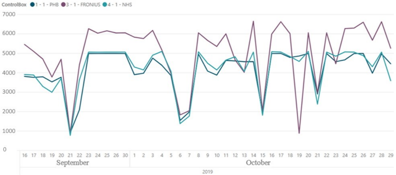
Fig. 11 Active power injected by inverters under control conditions.
