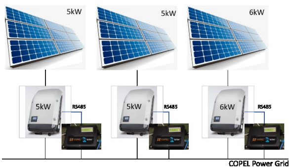
Fig. 9 Setup implemented for the test: inverter, photovoltaic panels (and its maximum power) and Control Box.
